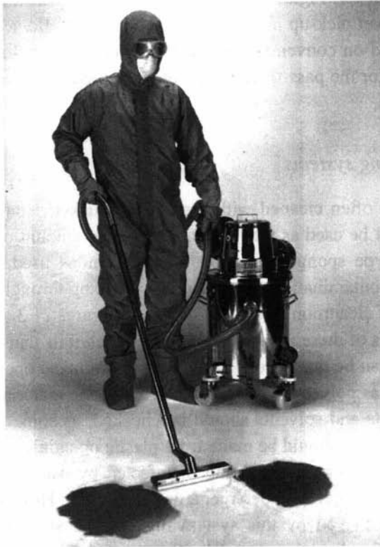
Figure 21.2 Vacuum system being used in its wet pick-up mode
