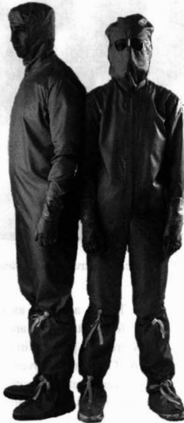
Figure 19.8 Cleanroom garments suitable for a higher standard of cleanroom
