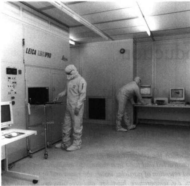
Figure 1.1 A cleanroom with personnel wearing special cleanroom clothing.
