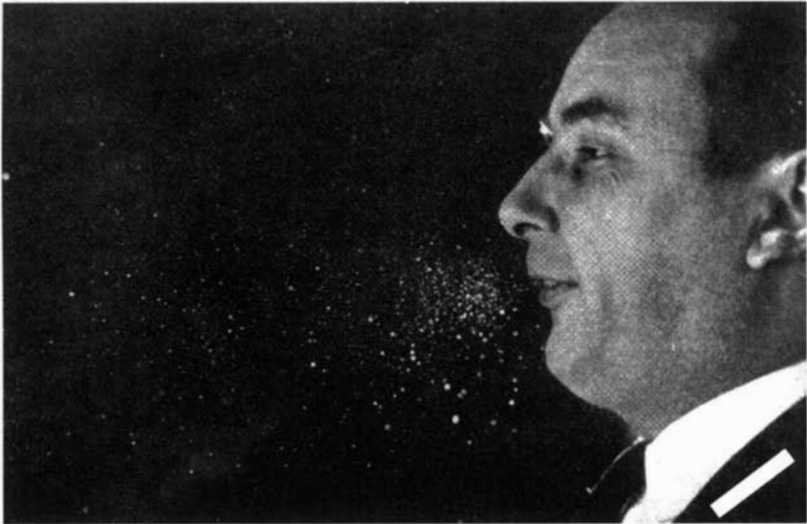
Figure 20.2 Particles emitted when pronouncing the letter 'f'
