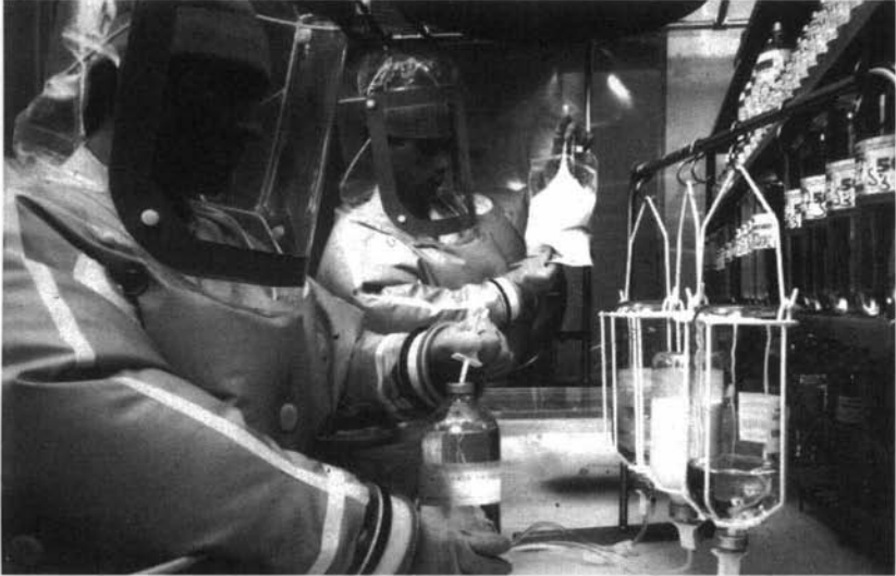
Figure 6.17 View of half suits and inside of isolator
