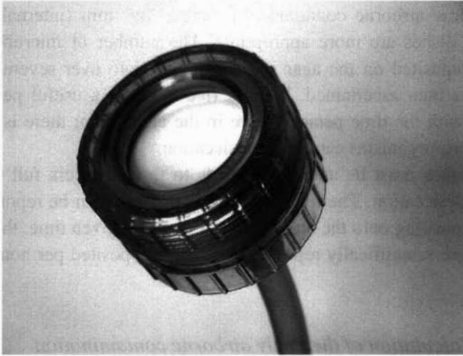
Figure 14.4 Membrane holder with filter
