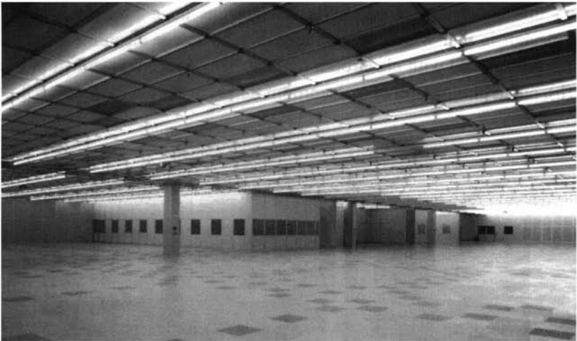
Figure 6.6 Ballroom type of cleanroom
