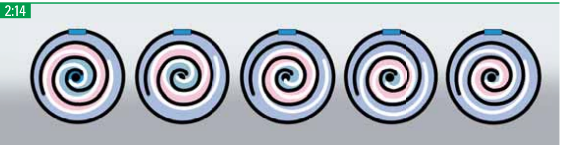
Compression principle of a scroll compressor.
