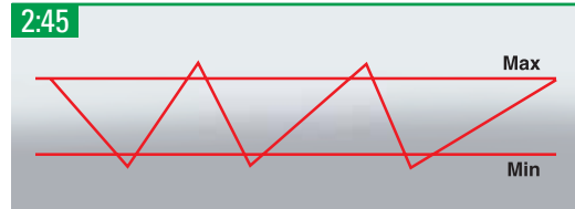
Pressure band, Min–Max, within which the compressor operates: "Min" = load, "Max" = off-load.
