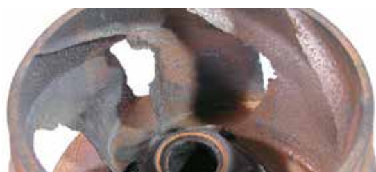
Erosion corrosion of cast iron impeller
