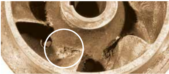
Cavitation corrosion of bronze impeller
