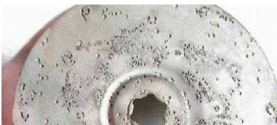
Pitting corrosion of EN 1.4401 (AISI 316)
