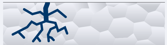
Fig. 1.6.10: Stress corrosion cracking
