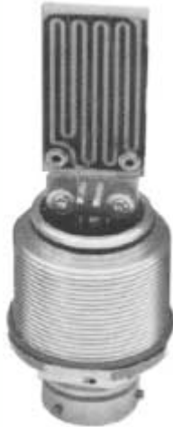
FIGURE 5.12 Thin-film resistor used for measuring humidity. (From Kreider et al., with permission)
