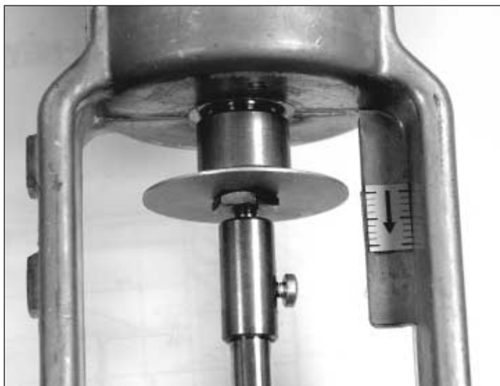
FIGURE 6.30 Picture of valve stem and position indicator.
