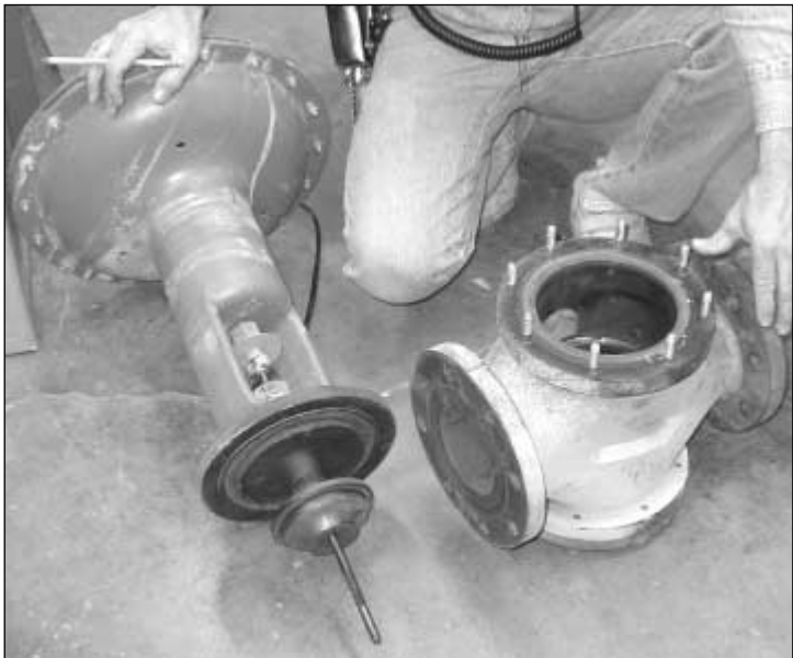
FIGURE 12.20 Six inch steam valve disassembled for rebuild.
