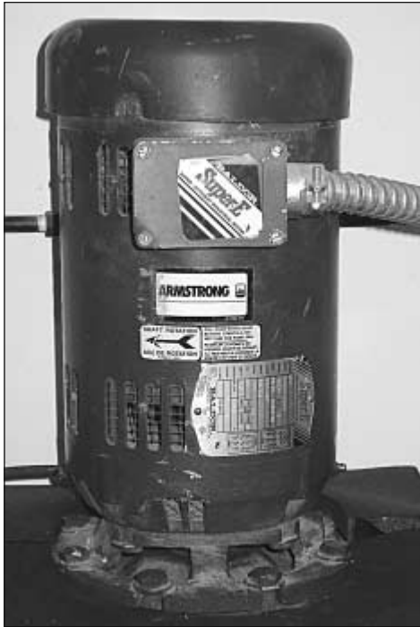
FIGURE 6.3 Close-coupled, sealed bearing pump.
