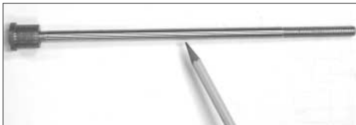
FIGURE 6.29 Valve stem showing area to check for wear.
