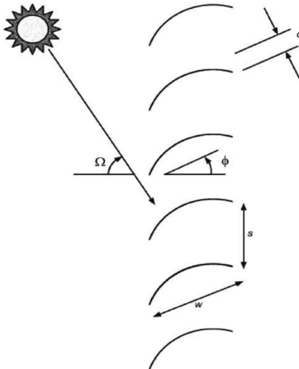
Figure 3.1 Geometry of Slat-Type Sunshades
