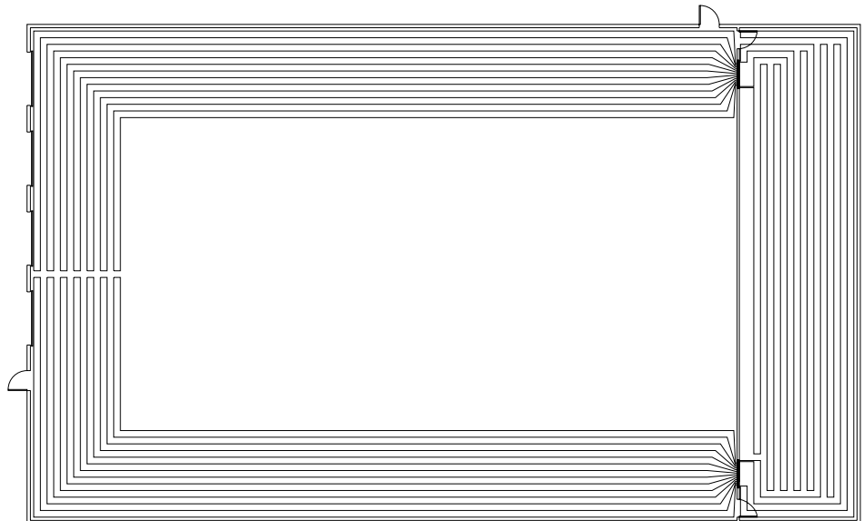
Figure 10-2: Full Coverage Tubing Installation
