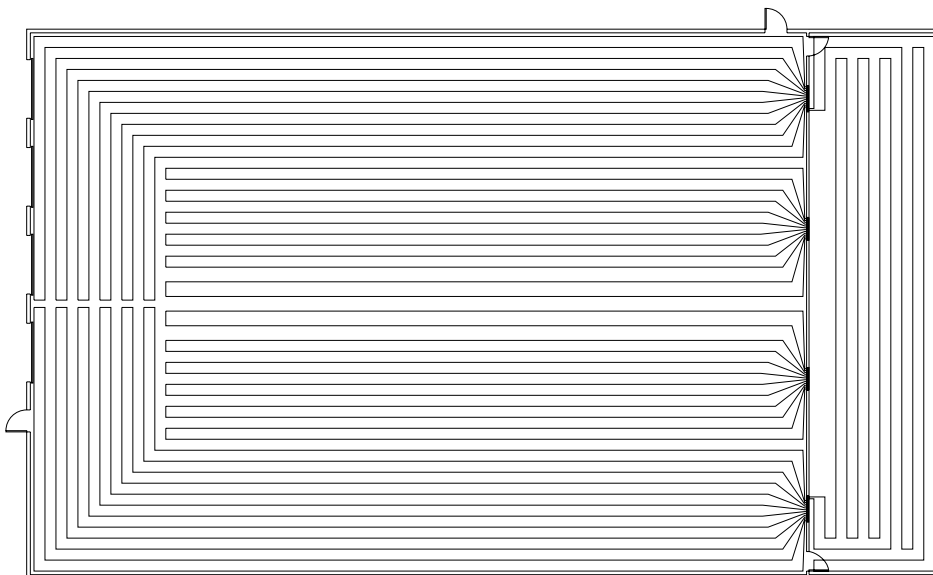
Figure 10-4: Varied Coverage Tubing Installation
