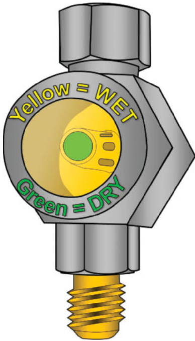
Figure 6–36 Sight glass with moisture indicator. Courtesy of Refrigeration Training Services.
