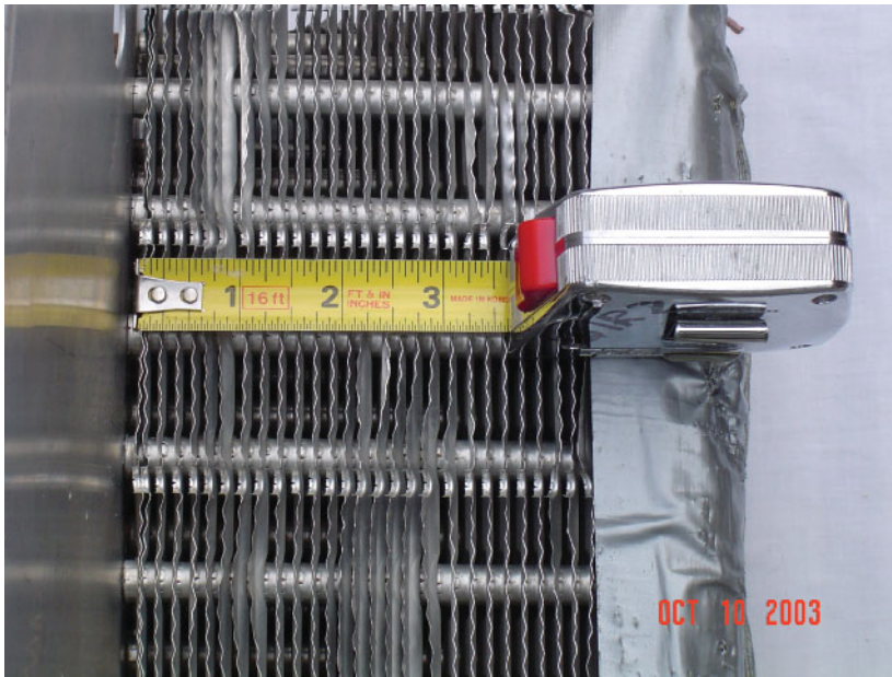
Figure 2–16 Measuring evaporator fin spacing. Photo by Dick Wirz.
