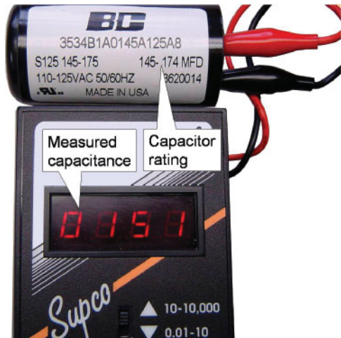
Figure 8–10 Checking a start cap. Photo by Dick Wirz.
