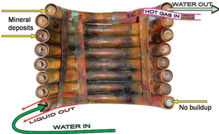
Figure 3–14 Mineral buildup in tube-in-tube condenser. Photo by Dick Wirz.
