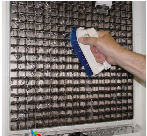
Figure 12–9 Use cleaner and a brush to clean ice machine evaporators. Courtesy of Manitowoc Ice, Inc.
