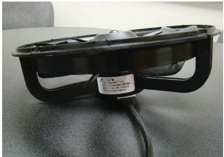
Figure 10–27 ECM evaporator fans. Photo
