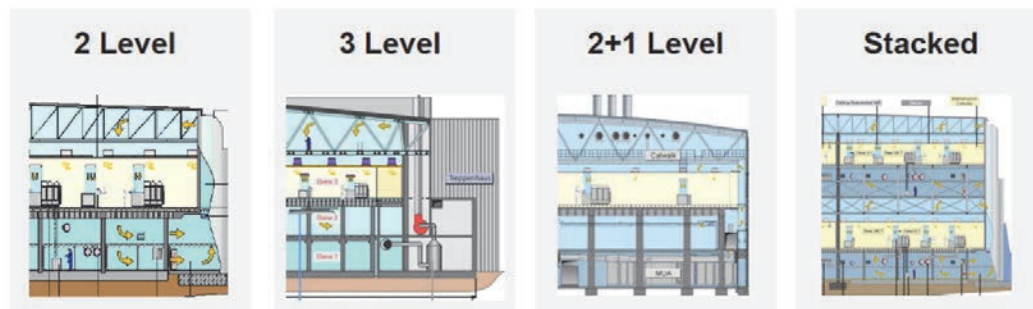
Figure 18.13 Multilevel Fab Options
